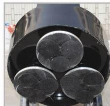
Planetary abrasive plate
